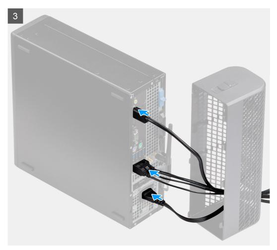
3. Align the cable cover retaining hooks into the slots on the Precision 3450 Small Form Factor chassis.
